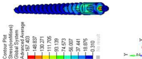
Fig 9: Von-Mises Stress in Miniscrew (MPa)
